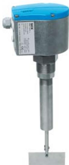
The MBA200 functions as a full, demand or empty indicator of bulk products in large storage silos as well as in small containers. In drop tubes and conveyor systems, the indicator provides a quick signal to indicate a blockage in product flow. One of the great features of the MBA200 is high reliability under most difficult operating conditions.
